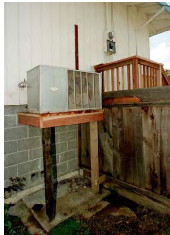
This house has an elevated air conditioning compressor and electric meter.
