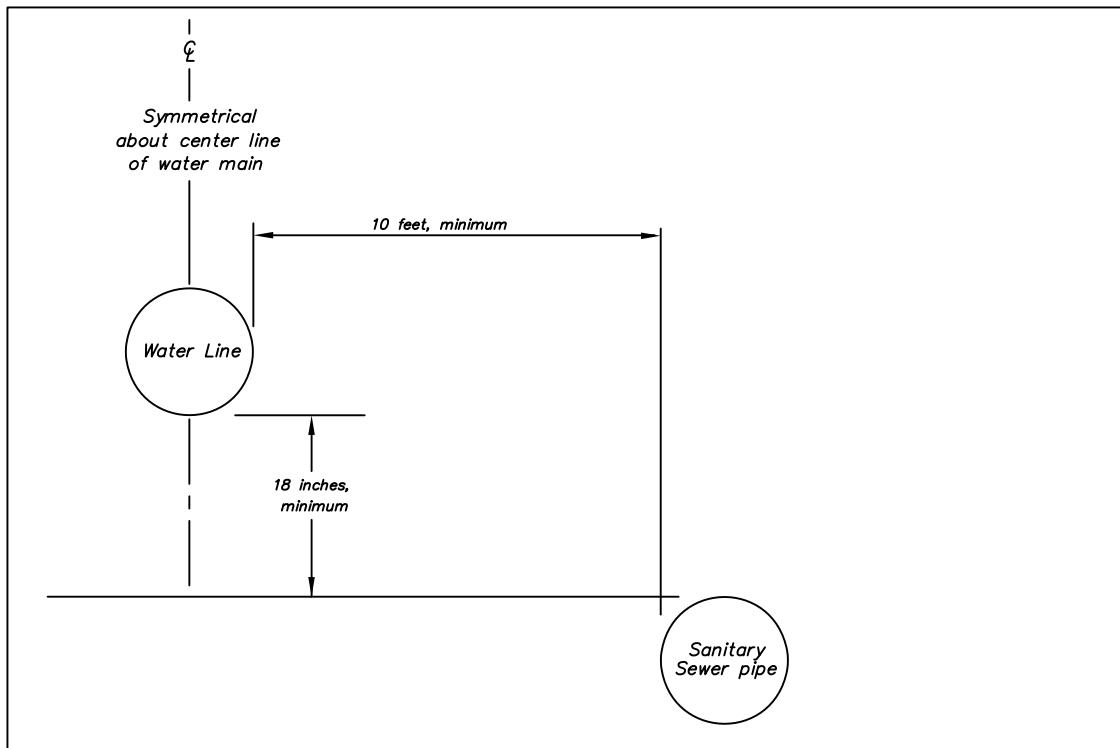
**Required Separation Between Water Lines and Sanitary Sewers, Unusual Conditions Parallel Construction**
