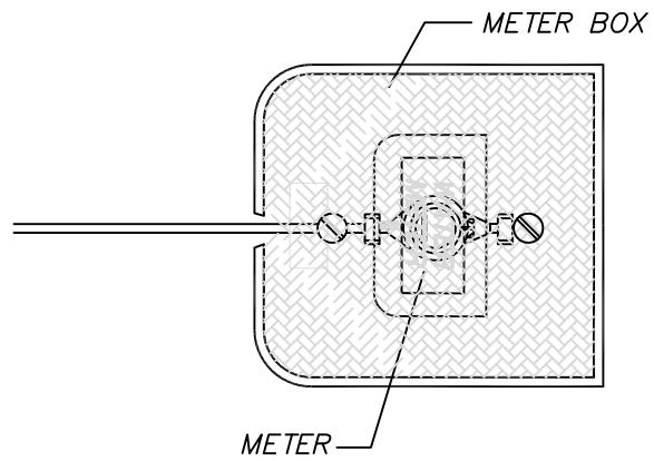
METER BOX - TYPE - Carson Heavy Wall as shown on the detail for specific meter size DUCTILE IRON COVER w/ FLIP READER LIDS, as shown on details All appurtenances placed inside meter box shall be centered to operate valves and read the meter.
